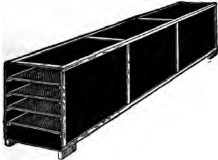
FIG. 15. Series of trays enclosed in wall-board box, for use with electric fan.
